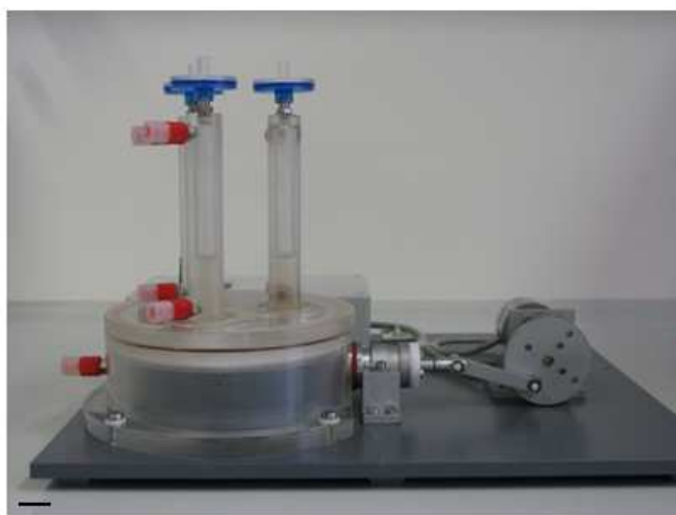
Fig 4. Pulsatile bioreactor. Comparison of different media, cells and scaffolds are enabled by three media compartments at defined mechanical loadings. Core unit manufacturing from acrylic glass provides optical transparency for macroscopical observation of processes within the unit (122). Scale bar = 20 mm.
